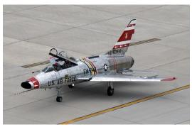
version of the Super Sabre. The last new-build version of the Super Sabre was the two-seat F-100F in 1957. Although intended to be a combat proficiency trainer, the F model could still carry two guns, 6,000 lbs. of ordnance and perform a variety of missions.
