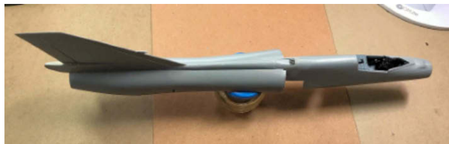
View of upper fuselage assembly, note the "coke bottle" shape that reduced drag at high speeds.
