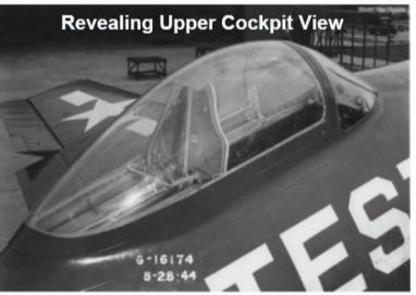
Although this is a B&W photo, Interior Green is clearly shown on interior canopy frame, seat, & deck. Black paint has been applied on the cockpit sides.
