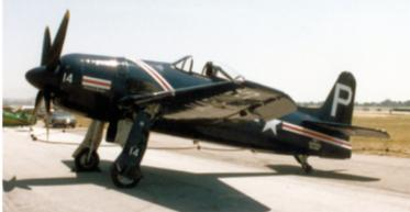
Left: Grumman's XF8F-1 "Bearcat" clearly designated for testing and, Right: Howard Pardue's restored F8F-1, with non-standard spinner hub, parked prior to some exciting airshow flying.
