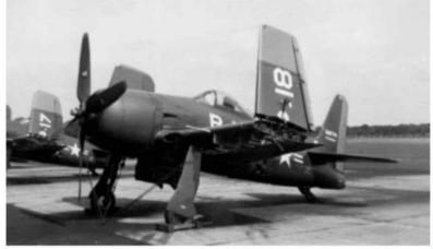
Uniquely marked and equipped F8F-2's with one (1) 20mm cannon per wing. Wings are folded.
