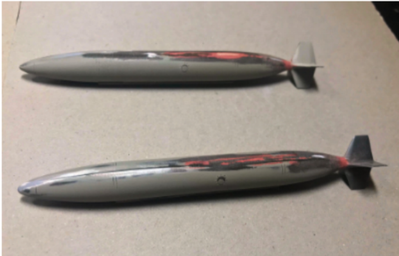
Custom wing tanks, primered, puttied, & sanded
