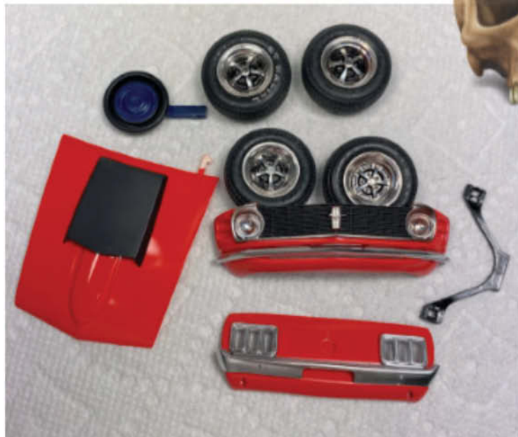
Grill, wheels, bumpers stripped of original chrome, then Alclad II Chrome was applied.
