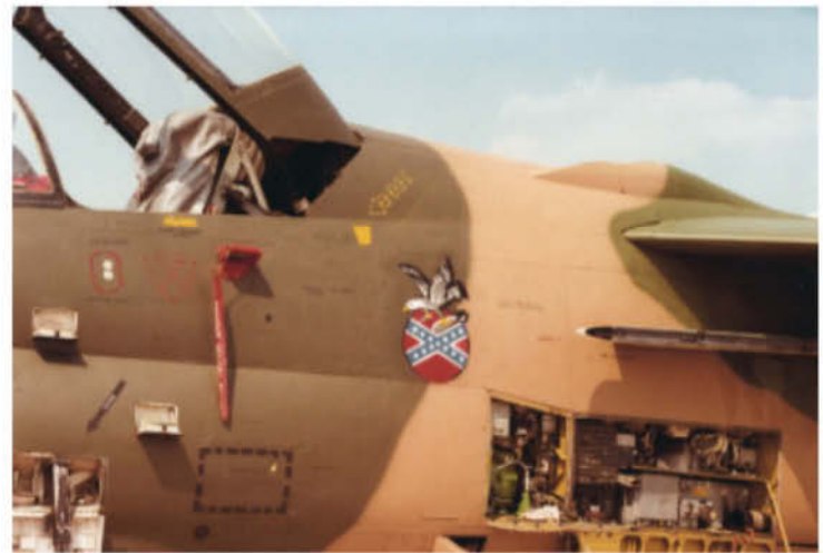
Detail of A-7D's forward fuselage with mostly subdued markings and open compartments.
