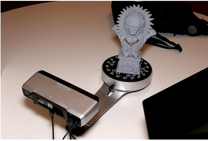
Part of Doug Hayes' presentation on scanning objects for 3-D printing and model making. John Mullins' bust is the subject set in place to be scanned.
